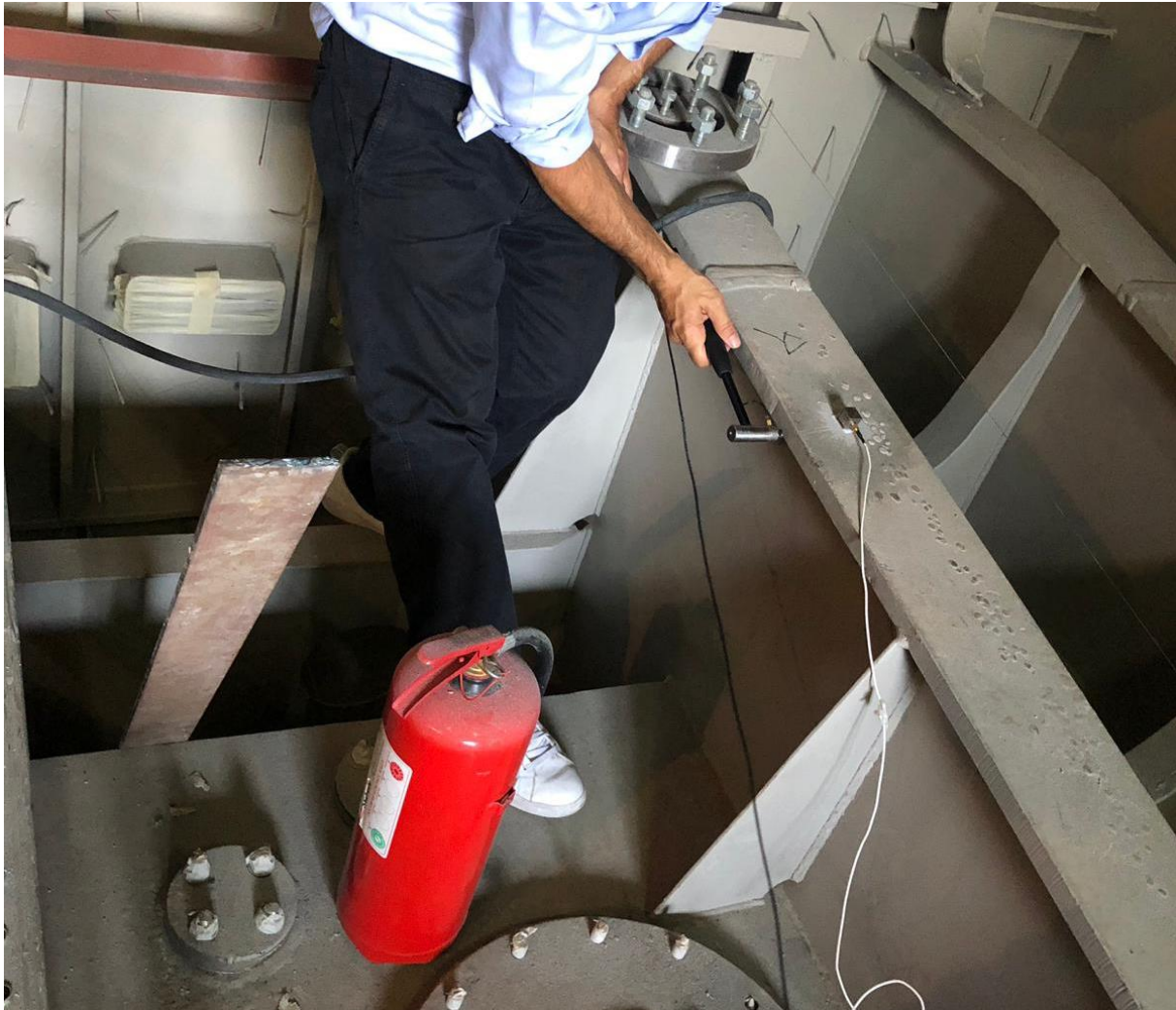
Figure 2. Impact testing in lateral direction of engine support structure.
