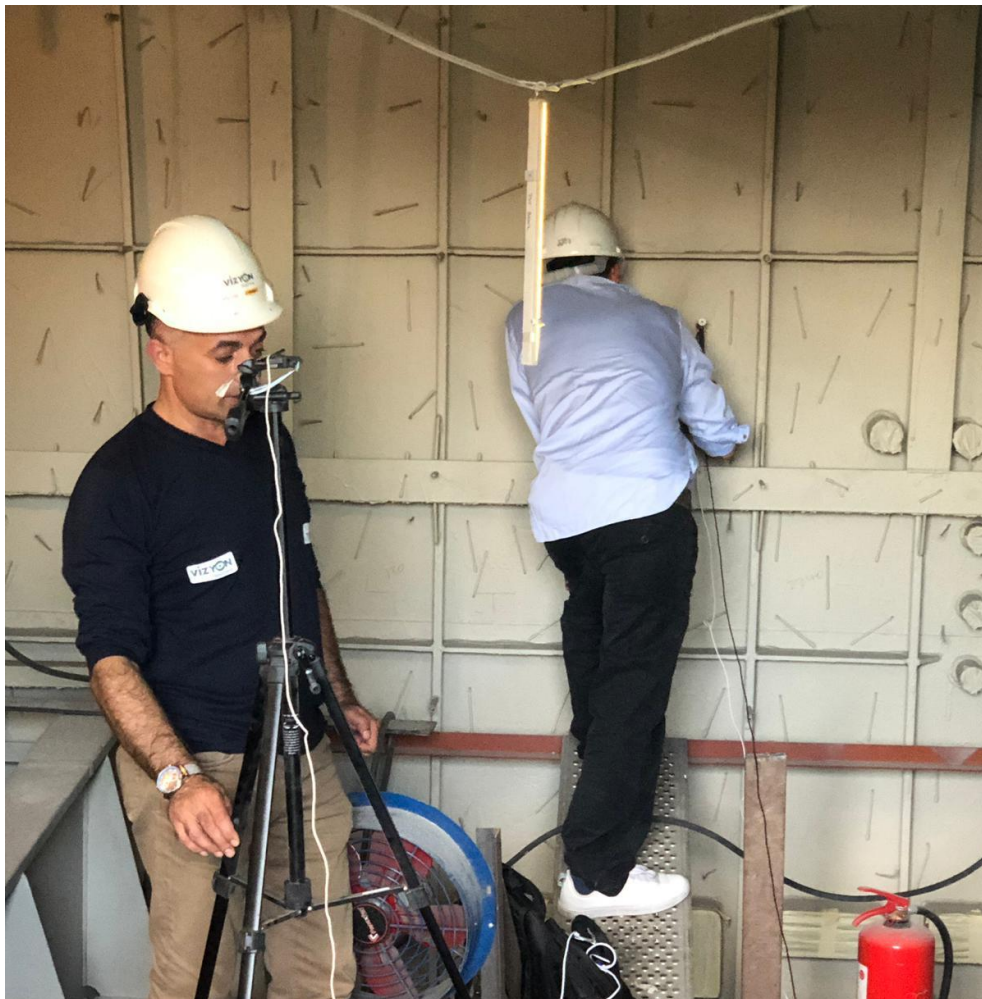
Figure 1. Impact testing in longitudinal direction of the yacht.
