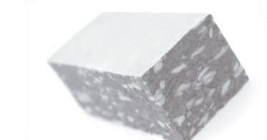
**Composition:** Fiberglass facing and bound polyurethane foam with a density of 150 Kg/m<sup>3</sup>.
