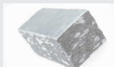
**Composition:** Aluminium facing with fiberglass support and bound polyurethane foam with a density of 150 Kg/m<sup>3</sup>.
