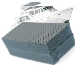
**Composition:** Beige perforated PVC facing, absorbing polyurethane foam and 5 kg/m<sup>2</sup> heavy viscoelastic mass inserted within.
