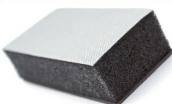
**Composition:** Fiberglass facing, M-1 class fire-resistant absorbing polyurethane foam and 5 kg/m<sup>2</sup>heavy viscoelastic mass.
